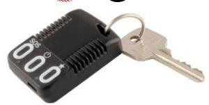
The TM-206 / R9D9 is a mid-range product line member of KCS' advanced TraceME track and trace modules. The TM-206 is targeted for remotely tracking and tracing a variety of objects, even livestock, and for personal use.
